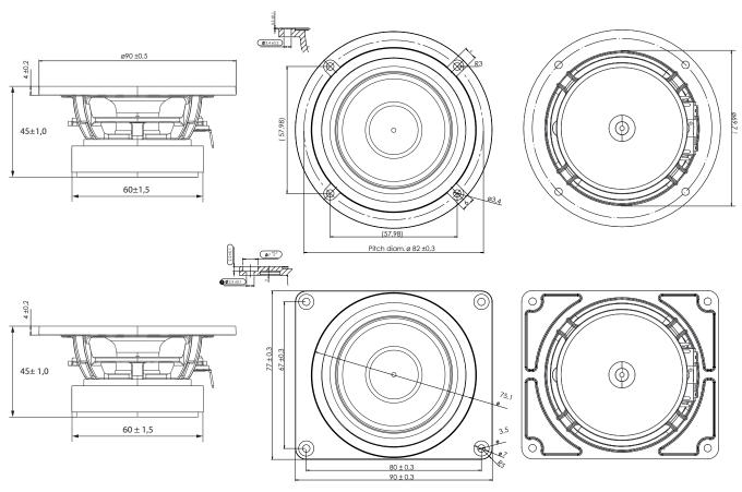
Note, since we now use a new factory and measuring conditions, the measures are updated. We also recommend paring drivers from the same factory. Please see our web site for replacement and upgrade policys. Measuring conditions: Factory new driver, not "broken in". Half space free-field (2 pi) above 100 Hz. Anechoic room 6x7x8 meters. IEC specs. refer to IEC 60268-5 third edition. All EAD products are RoHS compliant. Sensitivity/2.83V/1m/ 300-1000Hz.
