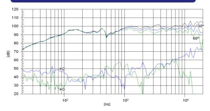
$\textbf{Note:} \ \ \text{Filtered frequency response measured with loudspeaker standing on infinite baffle in anechoic chamber, 1W @ 1m with FD-2XA and the standard of the standard o$
