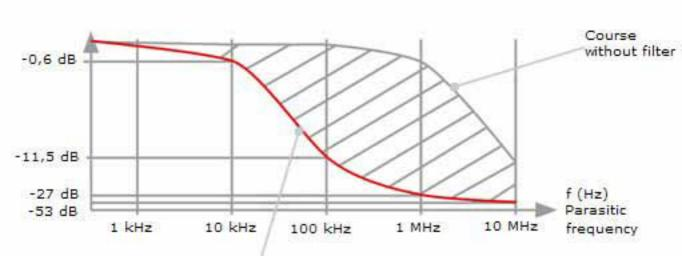
Course with special ferrite filter. Clearly visible is the suppression of high interfering frequencies.
