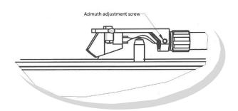
Having a correct azimuth setting maximises playback quality. Using the mirror from alignment tool "Align it" helps to find a correct setting - see following graphics:
