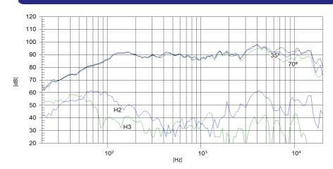
**Note:** Filtered frequency response measured with loudspeaker standing on infinite baffle in anechoic chamber, 1W @ 1m with FD-2CX/Fe
