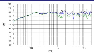
Note: Filtered frequency response measured with loudspeaker standing on infinite baffle in anechoic chamber, 1W @ 1m with FD-2XA
